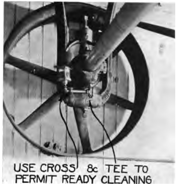
Fig. 2. Bearing equipped with Oil Cup.*
